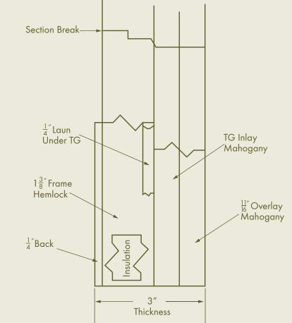
Pictured above is a cross-section from our custom wood garage doors! This drawing breaks down the composition of our 3" thick quality custom wood garage doors.
